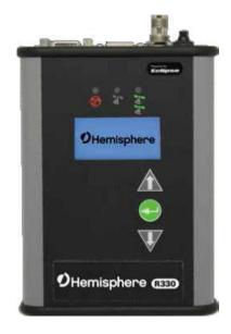
The R330 GNSS receiver is a full solution product in a compact enclosure. The R330 utilizes Hemisphere GNSS' Eclipse<sup>™</sup> platform and our latest GNSS patented technology. The R330 provides accurate positioning using several differential correction methods such as RTK, Atlas L-band corrections (H100, H30, H10), Beacon, and SBAS. Our patented firmware allows the R330 to smoothly transition between DGNSS systems.
